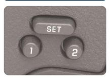
Your vehicle may be equipped with a two-driver memory function that is used to recall memory settings for the driver's seating positions for two drivers. The Driver Information Center (DIC) can also be programmed to personalize additional functions. See the DIC section of this guide for more details.
